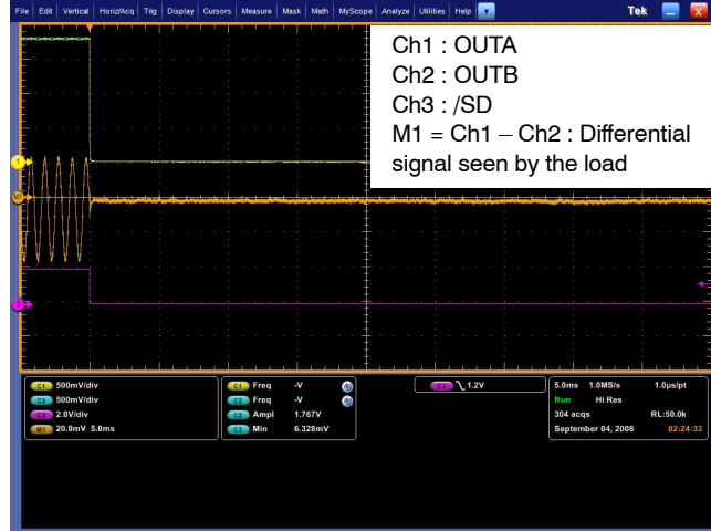
Figure 36. Zero pop noise turn off sequence with single-ended input audio source ( C_i = 47 \text{ nF} , R_i = 24 \text{ k}\Omega , R_f = 24 \text{ k}\Omega , C_{byp} = 1 \mu\text{F} , R_l = 8 \Omega , T_{on} = V_p )
