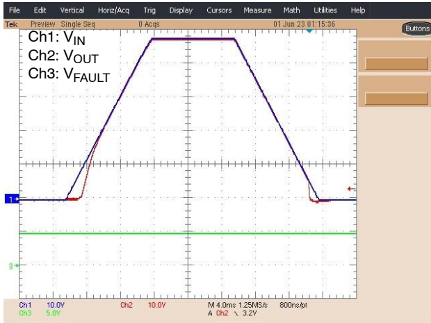
Figure 12. Turning on a Single Output with the Input Voltage (EN pin pull-up or floated)
