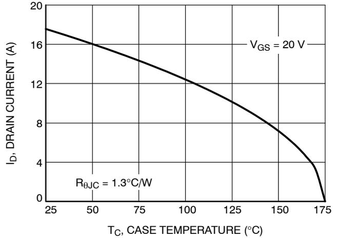
**Figure 11. Maximum Continuous Drain Current vs. Case Temperature**
