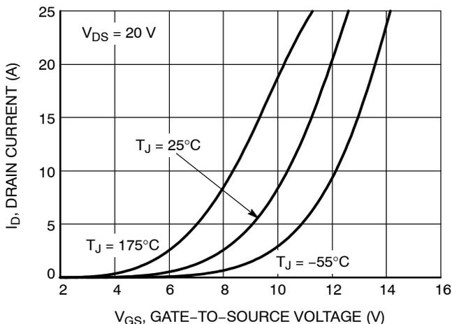
Figure 6. Transfer Characteristics
