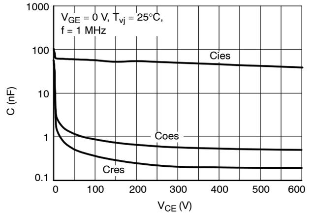
Figure 6. Capacitance Characteristic
