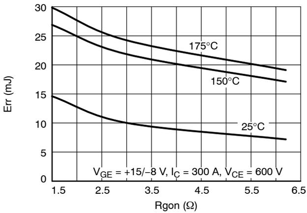
Figure 17. Diode Reverse Recovery Losses vs.  $R_{gon}$
