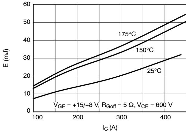
Figure 9. IGBT Turn-off Losses vs.  $I_C$
