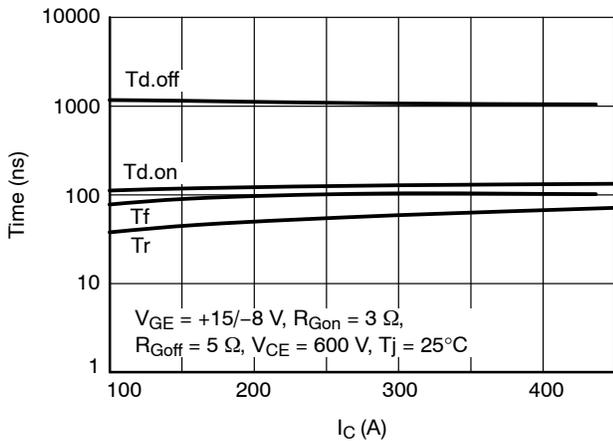
Figure 11. IGBT Switching Times vs.  $I_C$ ,  $T_{vj} = 25^\circ\text{C}$
