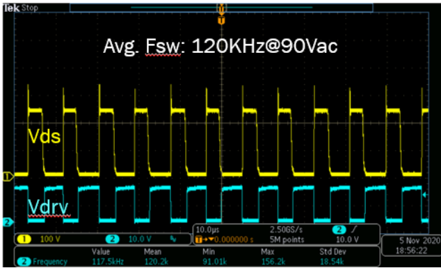
Figure 38. 90 Vac (CH1: Vds, CH2: Vdrv)
