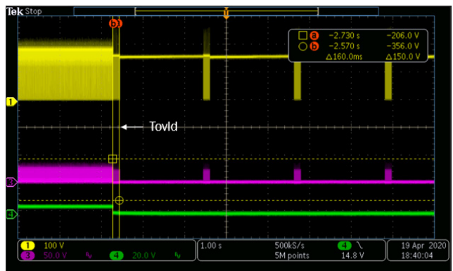
Figure 43. (CH1: Vdrain, CH3: Vsec-ds, CH4: Vo)
