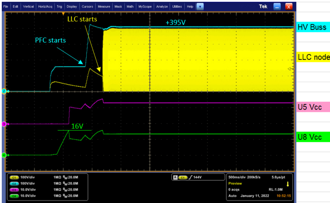
Figure 18. Power Supply Start-up Sequence
